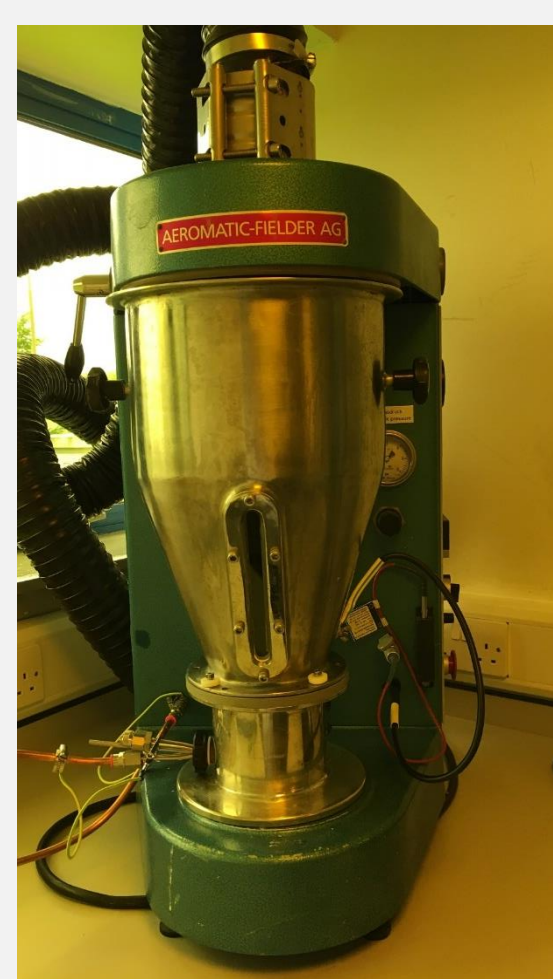
Figure 1 – Aeromatic Strea-1 coater with solvent coating capacity
